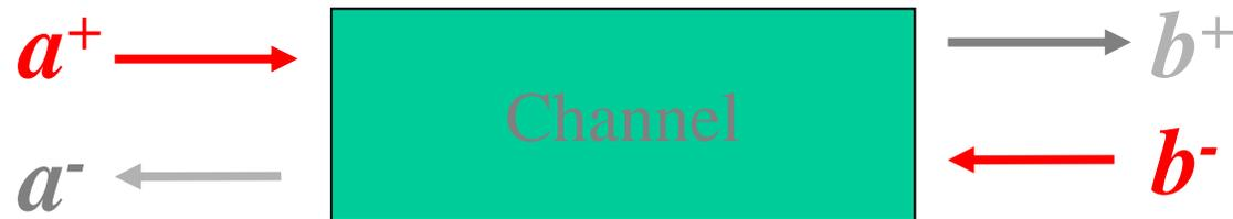
Usually we know  $a^+$ ,  $b^-$ . Coefficients  $a^-$ ,  $b^+$  and function inside the channel are unknown. To solve this problem we can use either **T-matrix** or **S-matrix** formulation.
